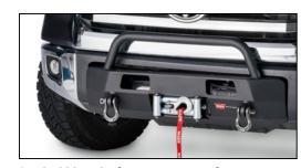
Semi-Hidden Kits feature open port for easy access to the winch clutch lever, and recovery points for mounting shackles (except Gen3 Tacoma)
