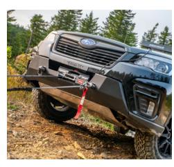
Semi-Hidden Kits for Subaru are compatible with winches up to 6,000 lbs. with mounting pattern of 3.0" x 6.59"
