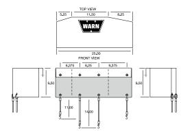
Fits the 16.5ti, M15 and M12 winches mounted on the Trans4mer, and Flatbed Mount 15639
