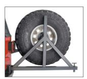
The WARN Tire Carrier for the Rock Crawler Rear Bumper is designed to carry a heavier wheel and tire, up to 37" in diameter. The carrier pivots on a robust 1–1/2" solid steel shaft pin that comes up through the bumper into the frame carrier. The shaft itself is welded – not bolted. Structural T-joint welds (vs. corner welds) will make this unit stand the test of time. A polyurethane pad reduces rattling. Includes frame reinforcing brackets.
