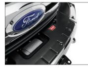
The Hidden Kit extends the original equipment Ford bumper out 8 inches. Winch controls to are easily accessed through openings in the top of the bumper.
